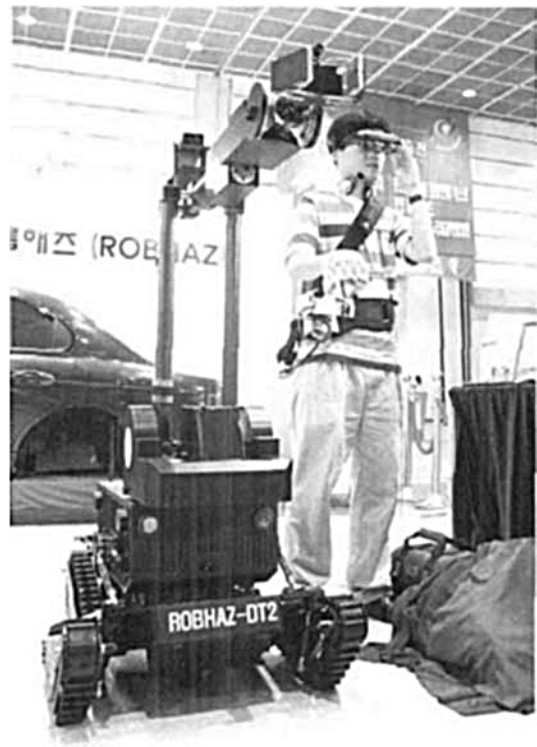
Fig. 5 Integrated field robot system: teleoperator with multi-modal interface and ROBHAZ-DT2
